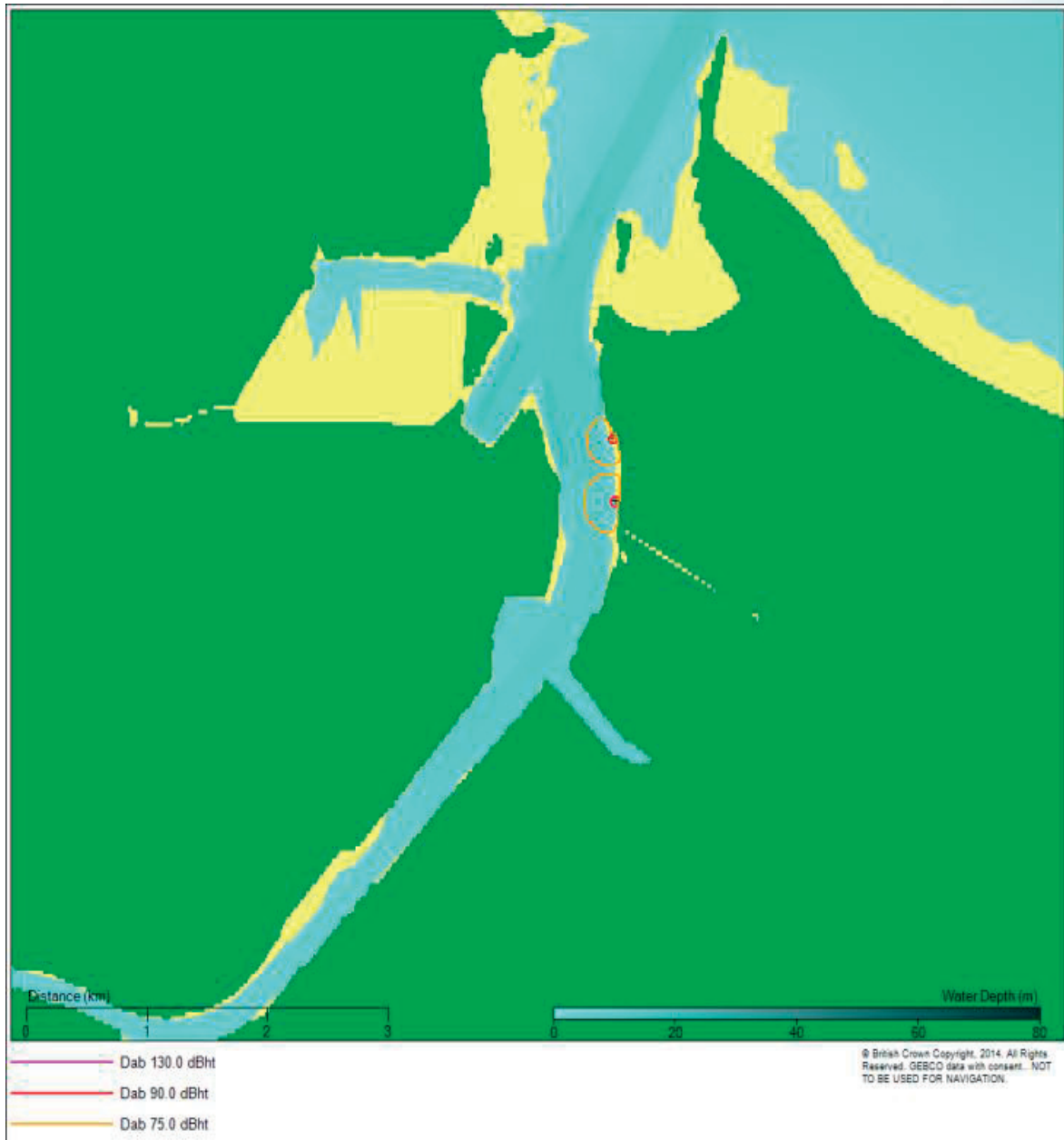
Figure 11-12 Contour plot showing the predicted 90 and 75 dB ht levels for dab for impact piling operations using a 914mm diameter pile and blow energy of 125kJ
