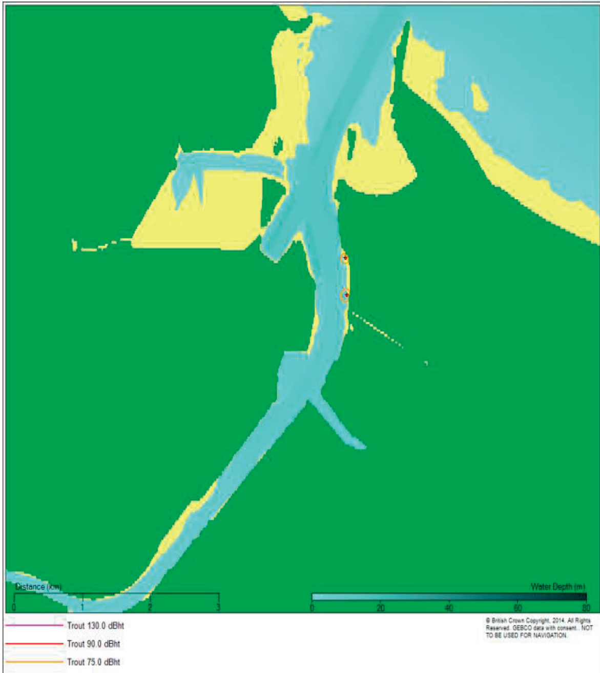
Figure 11-16 Contour plot showing the predicted 90 and 75 dB ht levels for sea trout for impact piling operations using 914mm diameter pile and blow energy of 125kJ
