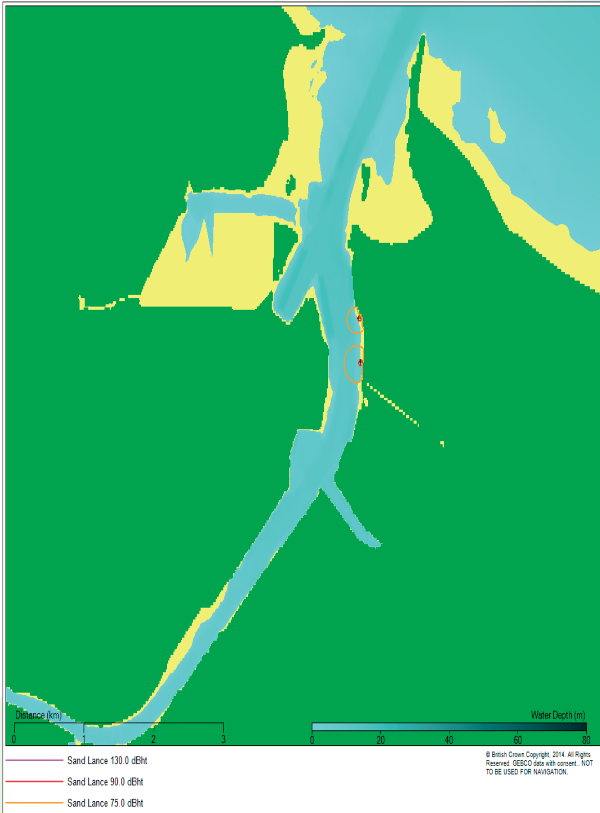
Figure 11-20 Contour plot showing the predicted 90 and 75 dB ht levels for sand lance for impact piling operations using a 2000mm diameter pile and blow energy of 305kJ
