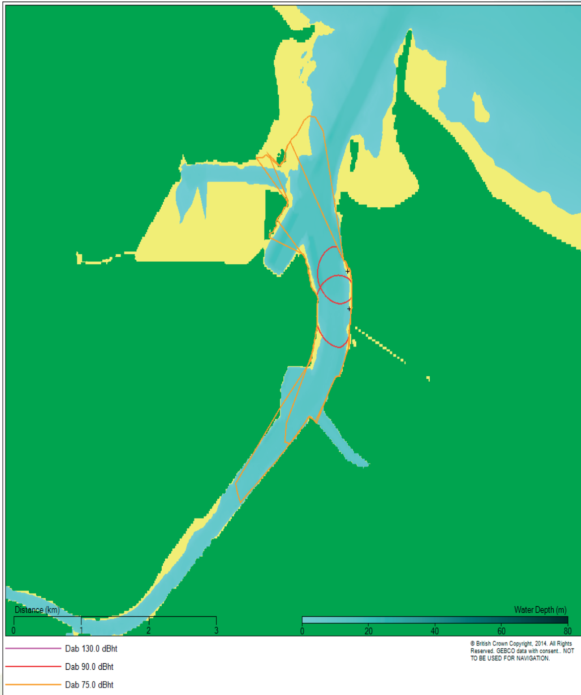
Figure 11-17 Contour plot showing the predicted 90 and 75 dB nt levels for dab for impact piling operations using 2000mm diameter pile and blow energy of 305kJ
