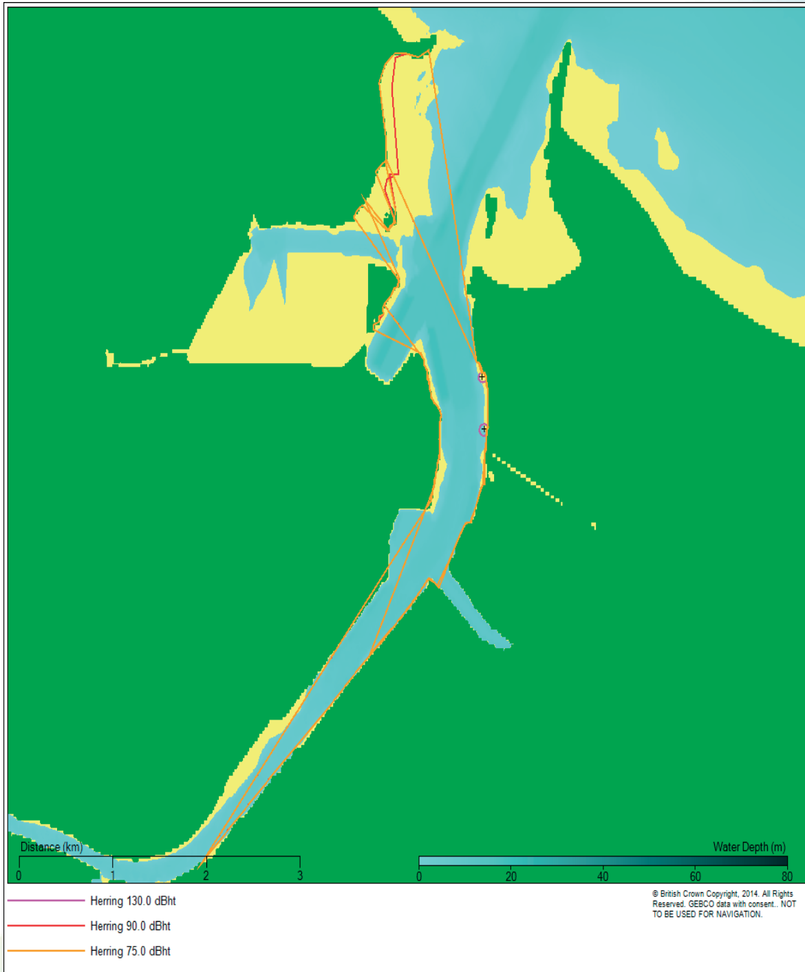
Figure 11-18 Contour plot showing the predicted 130, 90 and 75dB ht levels for herring for impact piling operations using 2000mm diameter pile and blow energy of 305kJ
