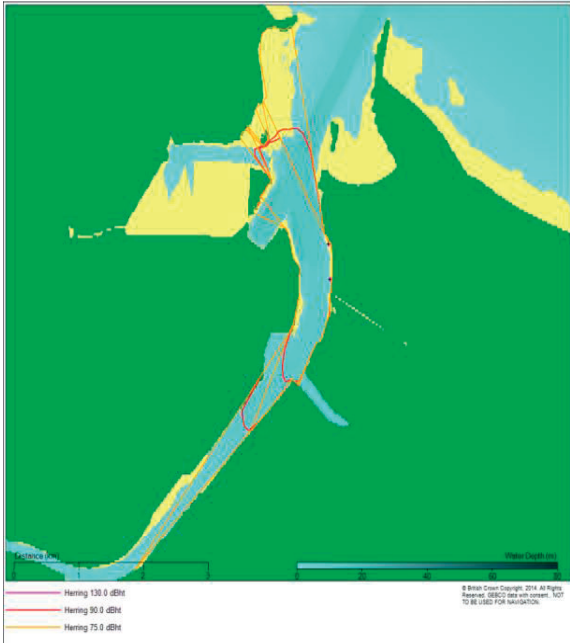
Figure 11-13 Contour plot showing the predicted 130, 90 and 75 dBht levels for herring for impact piling operations using 914mm diameter pile and blow energy of 125kJ
