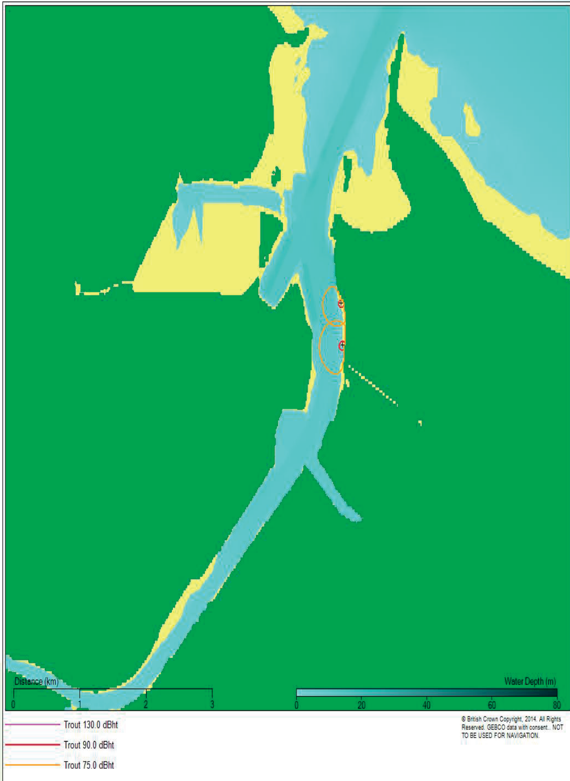
Figure 11-21 Contour plot showing the predicted 90 and 75dB ht levels for trout for impact piling operations using a 2000mm diameter pile and blow energy of 305kJ
