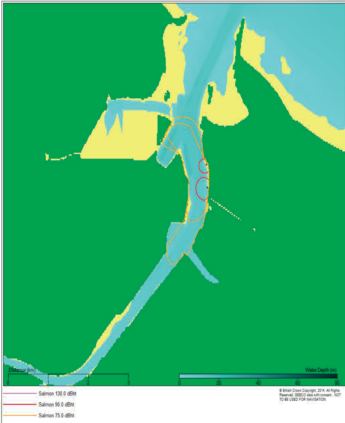
Figure 11-19 Contour plot showing the predicted 90 and 75 dB ht levels for salmon for impact piling operations using a 2000mm diameter pile and blow energy of 305kJ
