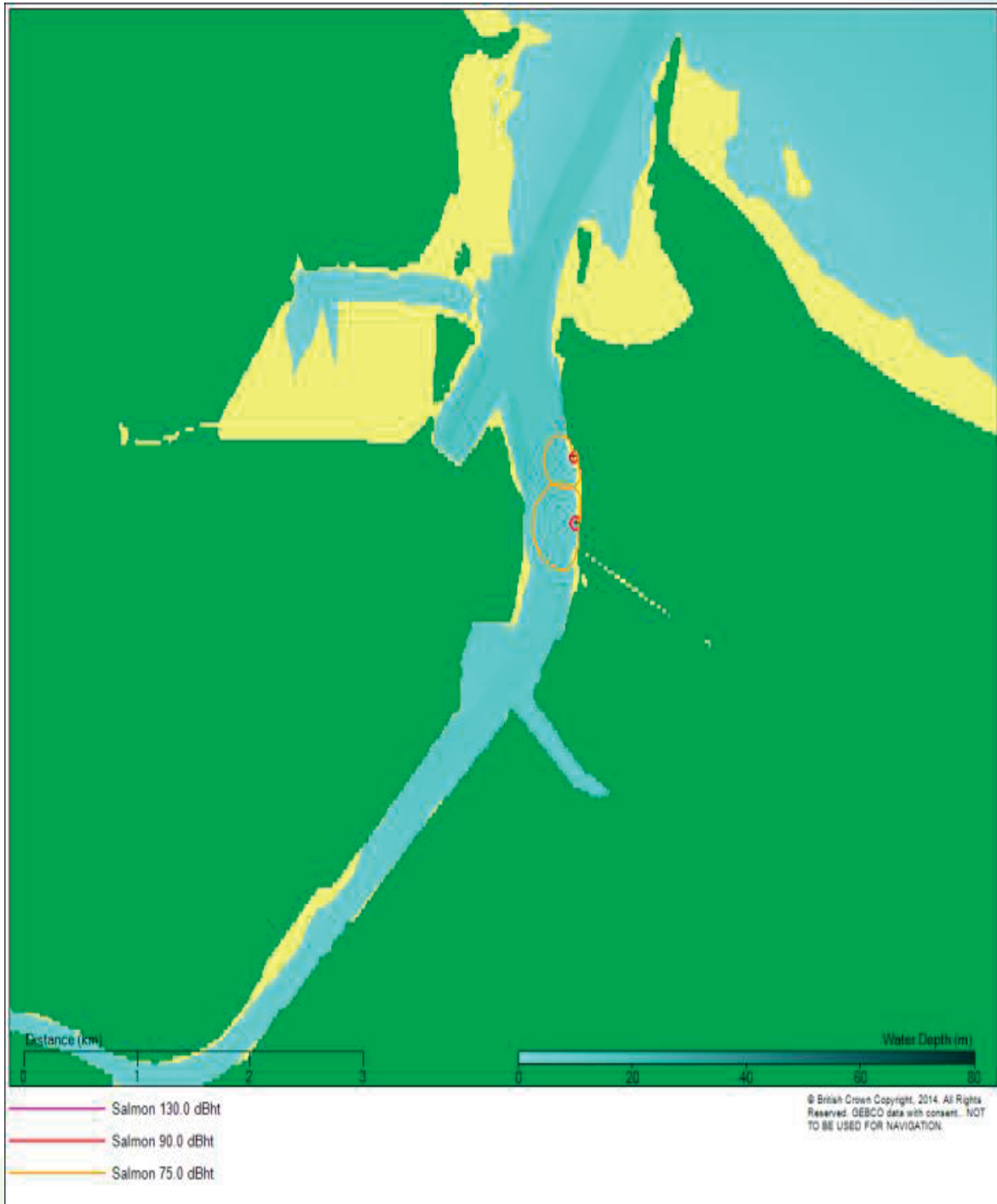
Figure 11-14 Contour plot showing the predicted 90 and 75 dB ht levels for salmon for impact piling operations using 914mm diameter pile and blow energy of 125kJ
