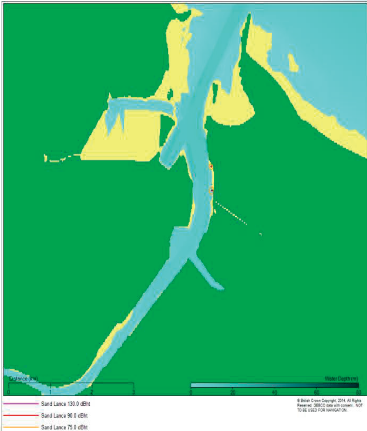
Figure 11-15 Contour plot showing the predicted 90 and 75 dB nt levels for sand lance for impact piling operations using 914mm diameter pile and blow energy of 125kJ
